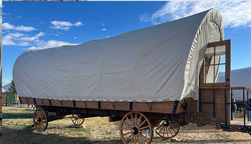
The second layer of vinyl canvas is stretched over the wagon hoops adding an extra layer of protection and making it easy to clean.
